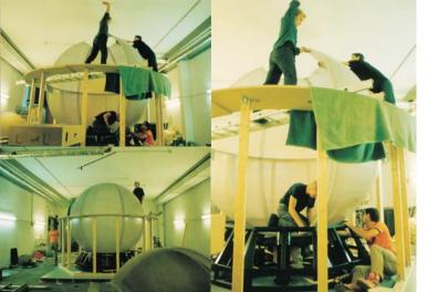
The segments of the sphere are constructed from a special plastic. The segments are attached to one another to form a three meter diameter sphere supported by the base. A removable pole cap is the entrance. The large ball lies on nine smaller balls, which themselves are mounted for freedom of rotation. In the base there is a brake ring and sensors to detect the motion
